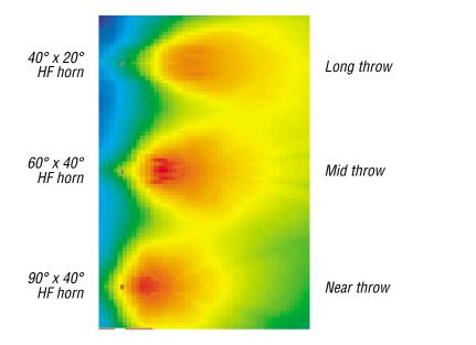
sound system design programs allow precise mapping of coverage of the horns to the seating while minimizing the sound spill (and feedback) to stage microphones and reflections from walls and ceilings.
