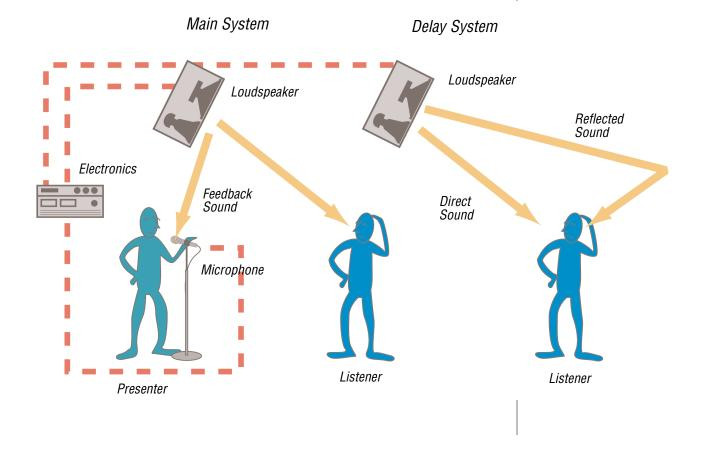
provides an important advancement in the performance of sound systems. DSP cannot only add delay but is also capable of adjusting the tone (equalization), limiting the loudness, act as crossovers, and even find and tune out feedback pitches. The application of DSP devices to loudspeaker systems gives the sound system designer the opportunity to use many different combinations of loudspeakers to provide fidelity and coverage for optimum sound in the worship environment.
