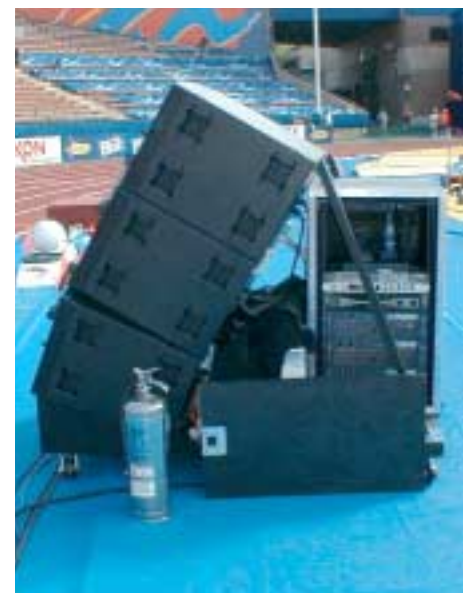
Closeup of the X-Line stacks with amps.
