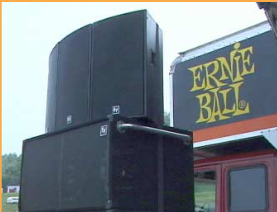
Three QRx-115 cabinets atop a MTL-1X 2 x 18-inch subwoofer in the left main array.
