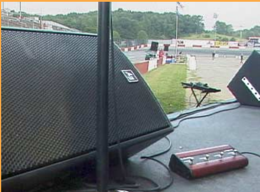
Two QRx 115s used as stage monitors. Note how cabinet geometry makes monitor use easy.
