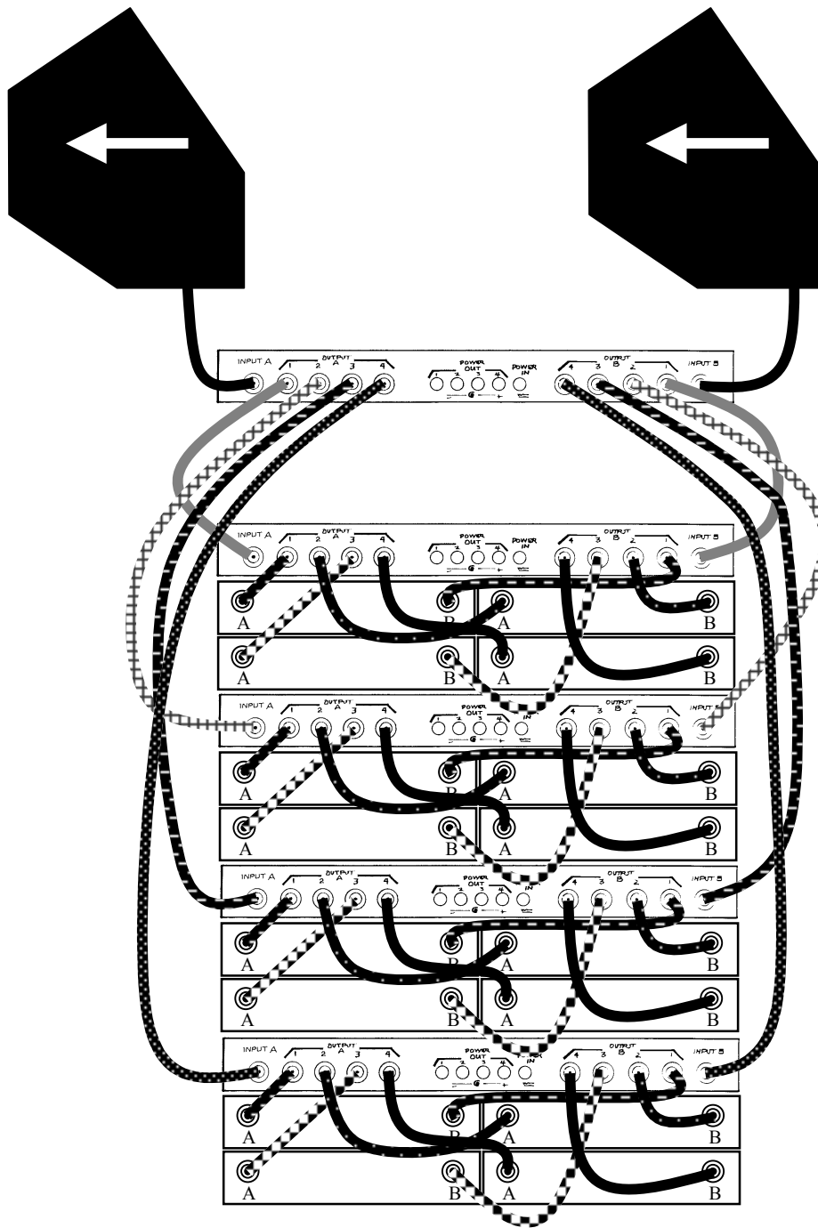
SIXTEEN RECEIVERS WITH FIVE SPLITTERS AND TWO ANTENNAS
