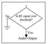
with a simple gate squelch is that any RF energy including distortion, hiss, harmonics from such sources as lighting dimmers, CD or DVD players, computers, digital effects and electric motors are indistinguishable from the desired signal. This extraneous RF energy will open the squelch gate just as easily as the intended transmitter. So often times the user must "crank" up the squelch level all the way up to limit the sensitivity to noise, which reduces range and performance of the system.
