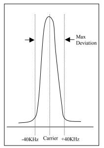
input into the microphone to generate 40KHz deviation. With the gain set above that we would be clipping or distorting the maximum input and if it is set too low we are not getting the clearest possible signal.
