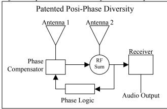
This process occurs in a fraction of a second and continually adjusts the phase of the second antenna for the optimum signal. A similar patented technique is used in cellular telephones to insure their reliable operation. Telex Posi-Phase diversity is more effective and less costly to produce than switching diversity because only one high quality receiver is required. Since only one receiver is needed, we are able to concentrate on the overall receiver design on more important aspects of the
