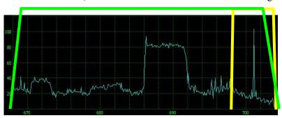
Telex introduced a unique solution to the front end filter problem in the FMR-1000/RE-1. These products include dual tuned filters that switch in where required based on the frequency of the signal. This approach allows a 24MHz (or 4 TV channel) wide operating bandwidth while using 12MHz filters. Dual tuned filters improve range and rejection which allows the RE-1/FMR-1000 to use 16 transmitters in 24MHz without any problems.
