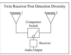
multiple receiver schemes, however there is a major drawback to antenna switching. The antenna switching receiver switches blindly, meaning that as the signal degrades, it switches to the other antenna even though the current signal may be the stronger of the two. The result can be a switch to a weaker signal, added noise, and possible dropouts. This is especially true at the edge of range.
