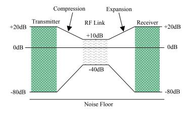
The compressor raises the average signal level above the noise floor to provide improved signal to noise through the RF link. The expander helps to reduce noise when the is no program content (a pause in speaking or singing) by suppressing any added noise as it restores the audio to its original dynamics.
