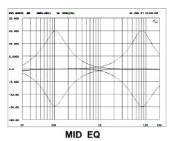
Adjustments in the MID range are certainly the most effective way to shape the sound. As a matter of fact, determining the correct center frequency is not always as easy as it seems. Here is one method – amongst others – how to quickly find the right setting of the parametric EQ for your application.
