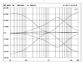
The HI and LO controls of the STEREO channels' EQ section provide a degree of control that is equally adequate for LINE level inputs and microphones. The MID control is active in a comparably wide frequency band around 2.4 kHz. With most microphones this is the critical range, where a slight attenuation offers excellent results.
