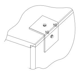
The FRi Series features internal heavy gauge steel reinforcing brackets that are not only designed to provide high safety factor support for the 3/8-16 forged eyebolt rigging, but also to unitize the internal panels for each enclosure. These corner braces are required to maintain the structural integrity of the cabinet to performance levels listed in this manual.
