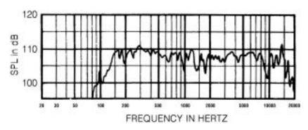
Figure 3—Axial Frequency Response Mid-Band Section only (1 watt/1 meter)
