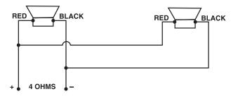
FIGURE 7 — Connection of Two EVM®10M Speakers in Series (net impedance is 16 ohms)
