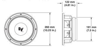
FIGURE 3 — Front Mounting Detail (not to scale)
