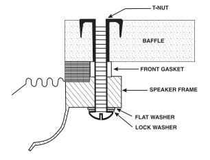
FIGURE 5 — Fillister and Internal Hex Drive Screws for Front Mounting (not to scale)
