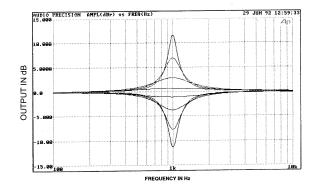
FIGURE 2 — Filter Response at ±12-dB Slider Positions
