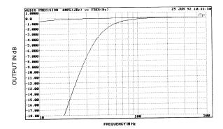
FIGURE 4 — Frequency Response, +6-dB Gain Position(high-pass filter off)
