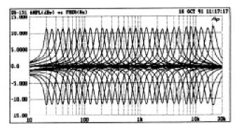
FIGURE 3 — Lo-Cut filter roll-off characteristics
