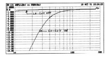
FIGURE 4 — EQ on, 12 dB range, ground switch "grounded"
