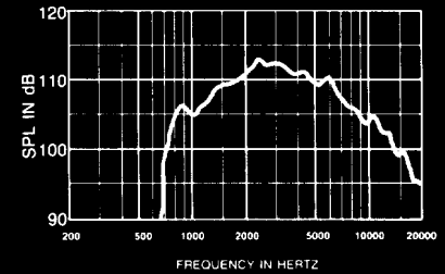
FIGURE 1 Axial Frequency Response 1 Watt/1 Meter Curved on HPT94 Horn
