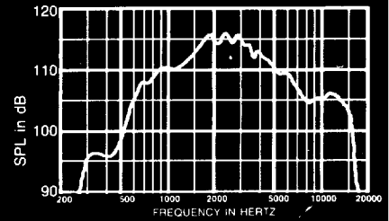
FIGURE 1 Axial Frequency Response, 1 Watt/1 Meter Curved on HP64 Horn
