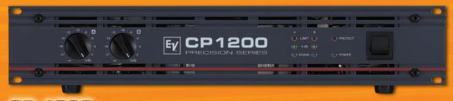
**CP 1200** With up to 2 x 600 watts into 2 Ohms and 2 x 400 watts into 4 Ohms dedicated for small fullrange cabinets and individual hi-frequency
