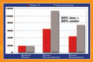
A conventional amplifier design has nearly double the power consumption and requires double the power dissipation over EV's Class-H Design of equivalent output power. The Precision Series Compact amplifier runs much cooler even under adverse conditions.
