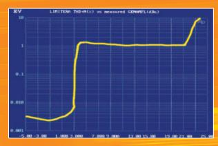
The THD of the amplifier is limited to a maximum of 1% for signals up to +21dBu. Even if overdriven, the amplifier will not create any objectionable "clipping signal effects" that are so fatal for speaker components.
