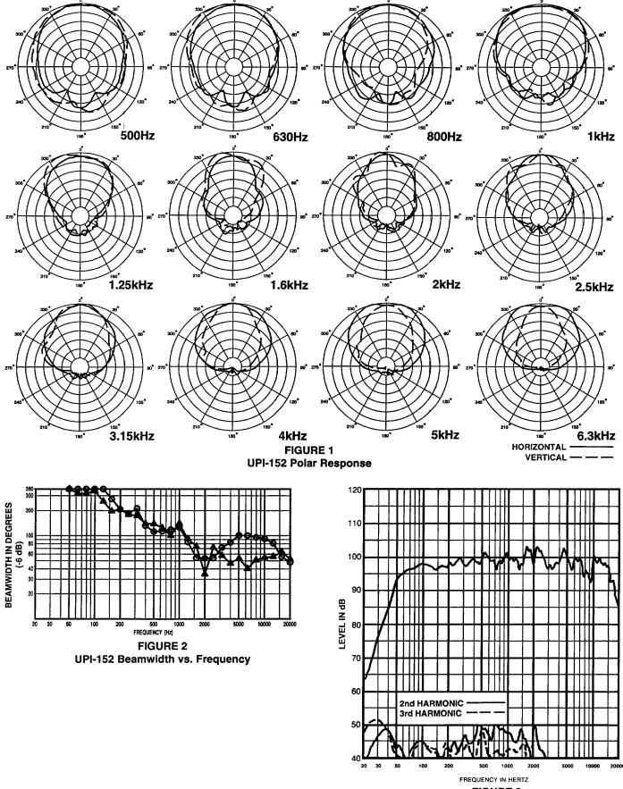
FIGURE 3 UPI-152 Frequency Response (1 watt at 1 meter)
