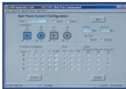
Software allows programming of pushbuttons and frequencies.
