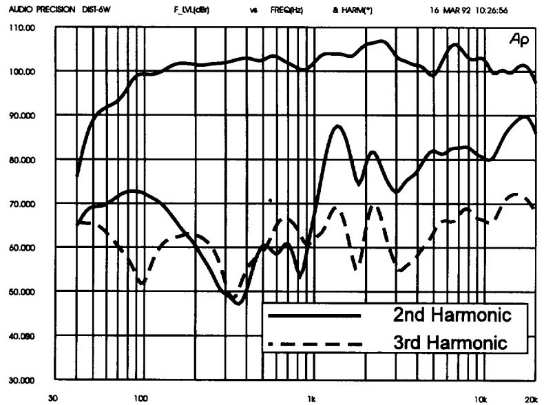
Figure 4—950-8B Harmonic Distortion at 0.1 rated power (25 W) 5
