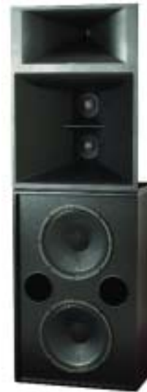
Variplex M-Matinee A 3-way system designed for mid-sized rooms providing all benefits of a three-way design, including the unique asymmetric directed coverage of all Variplex systems. Can be operated passive 3-way, biamp or triamp.
