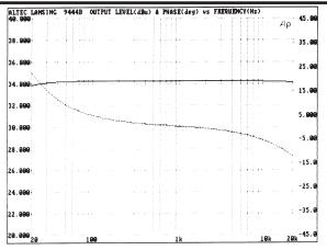
Figure 1. LEVEL (dBu) & Phase (deg) vs Frequency (Hz)
