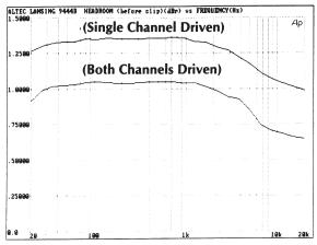
Figure 3. Headroom LEVEL (dBu) vs Frequency (Hz)
