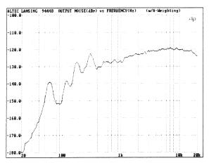
Figure 4. A-weighted Noise (dBr) vs Frequency (Hz)
