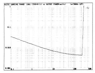
Figure 6. 1 kHz (THD+N) (%) vs Output Power (W)
