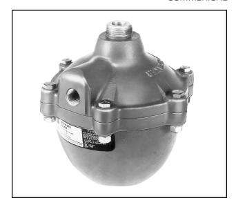
The driver voice coil impedance shall be eight ohms (16 ohms on the 7110XC-16). The internal driver will employ a linen-based, molded phenolic diaphragm, 11/2-inch diameter voice coil and "rim-centered" ferrite magnet structure. Replacement part 353 voice coil (439 for the 7110XC-16) and diaphragm assembly shall be available.
