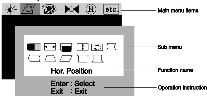
3. Press  $\leftarrow$  or  $\rightarrow$  to locate the function item. Then press **Enter** and  $\leftarrow$  or  $\rightarrow$  to make the adjustment.
