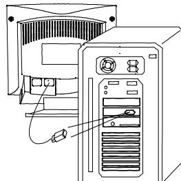
*If you connect the monitor to an Apple Macintosh through a D-Sub cable, you need to buy a Macintosh adapter to connect the video signal port of your computer and the monitor signal cable.*
