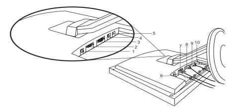
B. Connect the signal cable to the VGA output of the graphics card on the computer.
