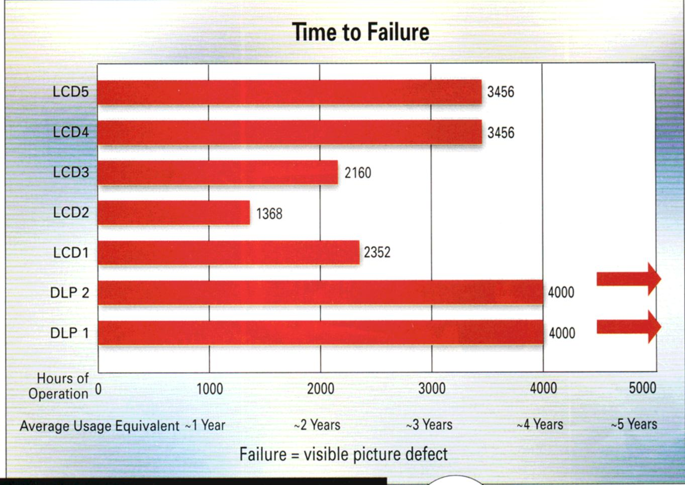
In the MCSL tests, DLP™-based projectors performed for over 4000 hours with no degradation, greatly out-performing LCD-based projectors
