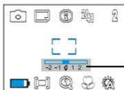
An exposure value bar will appear on the LCD monitor after pressing the "Right" and "Left" navigation button, you can choose to increase or decrease the exposure value of taking photos by using the navigation buttons.
