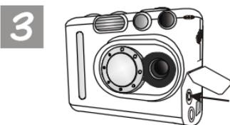
After opening the A/V out cover, you will see the A/V output port as the arrow shows.
