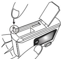
Open the cover. Then press down the elastic bar beside the memory card socket until the bar is fixed.
