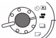
Push and adjust the switch dial to video mode on the top of the camera. Then the video mode will be activated. When video mode is activated, the icon
