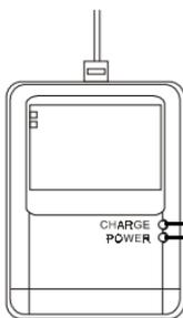
Then connect the power cord to the power outlet and you will the "CHARGE" indicator on the charger become red. This means the charger is charging the lithium battery.
