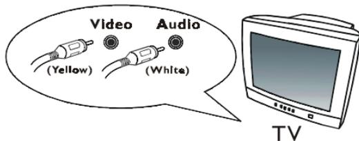
Then connect the other two ends of the TV cable to the Audio input port and Video input port of your TV. Please note that the yellow header is for Video port and the white header is for Audio port. After the connection to your TV, you will see the LCD monitor function on your TV screen.
