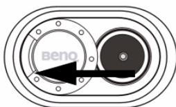
Slide the lens cover in the direction shown and turn on the power.
