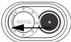
To turn on the power, you have to slide the lens cover in the direction shown. You will see the LCD screen show a frame of Benq logo. Then this camera is ready to work.
