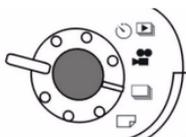
Adjust the switch to burst mode on the top of the camera. Then the burst mode will be activated. When burst mode is activated, the icon
