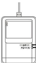
Then connect the power cord to the power outlet and you will see the "POWER" indicator on the charger turn in red. This means that the DC 3310 is ready to work.
