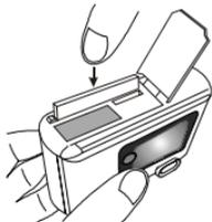
Place battery in the battery compartment and then press down the memory card into the socket until it is firmly fixed.
