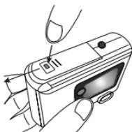
Press the PUSH button on the battery cover and then slide the cover in the direction shown.
