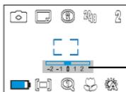
An exposure value bar will appear on the LCD monitor after pressing the "Right" and "Left" navigation button, you can choose to increase or decrease the exposure value of taking photos by using the navigation buttons.
