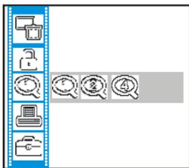
**2** Then press the right navigation button to select the zoom-in rate you want. There are three rates-1X, 2X and 4X for you to choose. The image will be zoomed on the LCD display. You can press Disp/OK button to change setting and also the right and left navigation button to adjust the position of the image you want to see.
