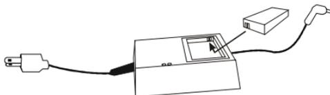
Put the lithium battery in the direction shown above and make sure the "+" and "-" contact parts are put in the right direction.
