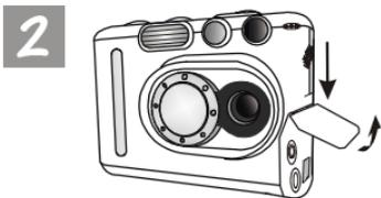
Slide the A/V out cover and open it in the direction shown.
