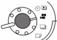
Adjust the switch to video mode on the top of the camera. Then the video mode will be activated.
