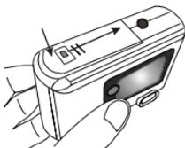
Close battery compartment cover and slide the cover in the direction shown. You will hear a click sound when the cover is firmly closed.
