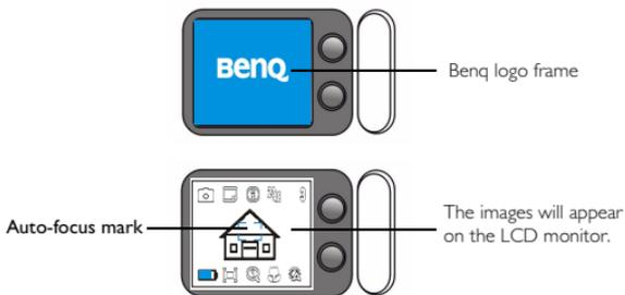
The image will appear on the LCD monitor and you will see a blue auto-focus mark in the center of the LCD monitor. Move the camera until the image on the LCD monitor is on the desired position.
