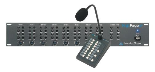
The DigiPage Jr is a matrix switching system allowing any one of up to 8 remote paging microphones (DPJ88M) to page into any combination of up to 8 output zones over industry standard CAT-5 cable. The system also allows any one of up to 4 program inputs to be directed to any or all of the 8 output zones. An emergency input is also provided.
