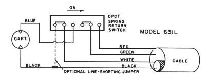
The model 631L may be rewired in the field. If a line-shorting function is desired, remove the rear housing and add a jumper wire as indicated
