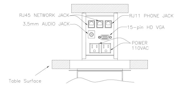
NOTE: A typical connector installation is shown in the above diagram. Various combinations of connectors, along with the applicable cable types, may be selected for customization at the time of purchase.
