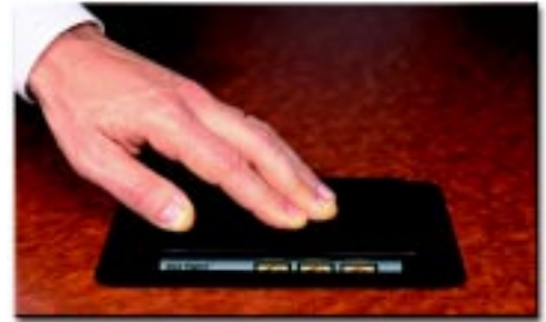
The top panel of the PNP202 requires 7 lbs. of pressure to release its internal electromagnetic locking mechanism, making it easy to pop up while avoiding undesired activation by light-weight objects.
