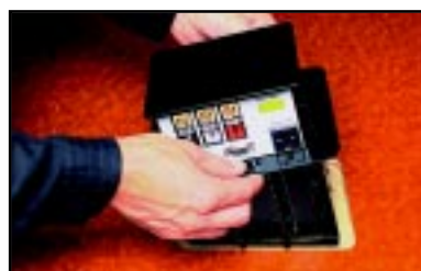
Place PNP202 tower into cutout.
