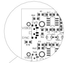
Set the VIDEO/SYNC switch to match the type of output signal being used.
