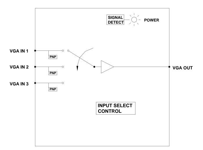
MT104-105 3 IN, 1 OUT VGA SWITCHER + 350MHZ + SIGNAL DETECT
