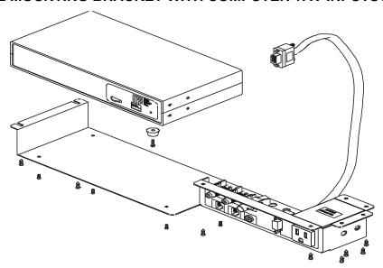
The TM1274 mounting bracket has the same capabilities as TM1273 with the addition of an AC Power connector.
