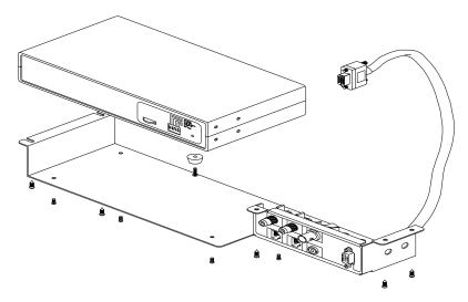
The **TM1273** mounting bracket, in addition to computer video input also offers composite video, audio, computer audio, telephone, and LAN connectivity.
