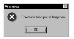
The screen above shows that some other program is using RS-232 port. If this happens close the program that uses this particular Com port and try again. Keep in mind that the software is switched into demo mode and you may have to select the set up tab and set the port to the required Com port.
