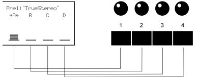
When in Program Edit Mode or Mix Edit , the Quad Knobs are linked to the parameters that appear in the right side of the display. The lower line of the alphanumeric display will show the abbreviated name of each parameter, with a bar graph below it representing the current setting of the parameter. By turning Quad
