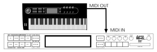
The MIDI THRU jack carries a replica (or echo) of the signal appearing at the S4 Plus' MIDI IN, allowing you to trigger other devices from the same controller which is feeding the S4 Plus. Simply connect the S4 Plus' MIDI THRU to the other device's MIDI IN. Note that the MIDI THRU jack will not send messages from the S4 Plus' keyboard itself.
