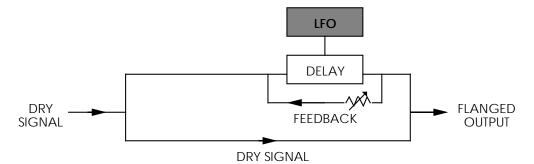
Many variables are available, from varying the speed and depth of the LFO to feeding back part of the signal to make the effect stronger. The Flanger's waveform shape can be either "Normal" or "Inverted". Use the "Inverted" setting for a more dramatic flange effect.
