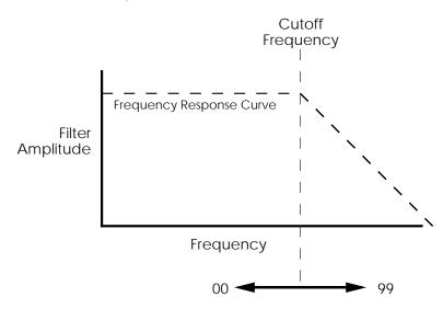
The cutoff parameter changes the frequency at which the highfrequency response starts to roll off. Lower values give a lower cutoff frequency. A value of 00 will cut all sound off.
