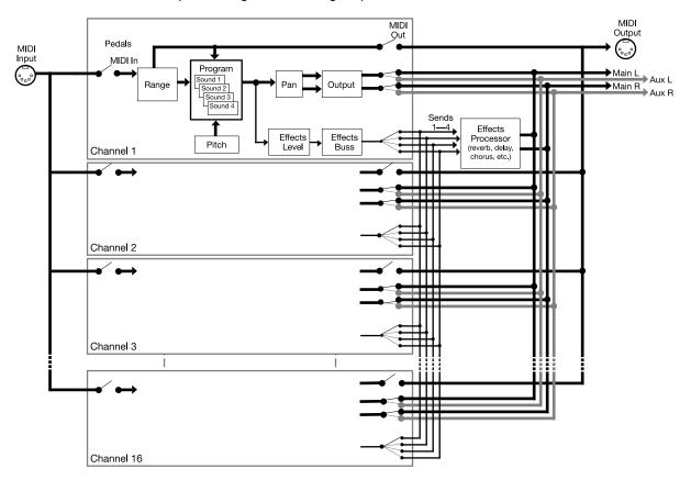
Here is a simplified diagram of the signal path in Mix mode.
