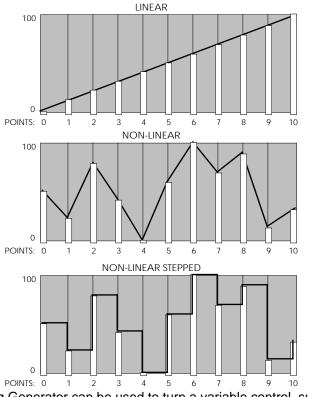
*Tip:* The Tracking Generator can be used to turn a variable control, such as the Mod Wheel or velocity, into a switch by setting all of the points to 0 except for point 10. Only near the maximum input will anything other than 0 come out of the Tracking
