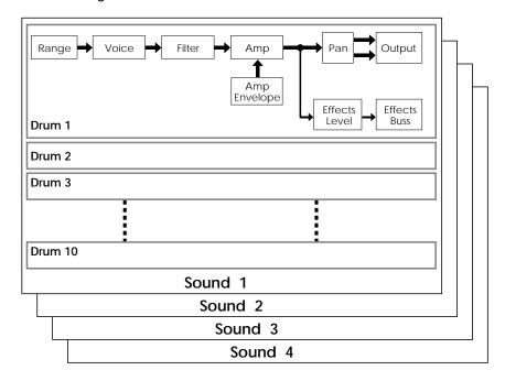
Here is a block diagram of a sound in Drum Mode.
