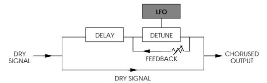
**Stereo Chorus.** In the case of a Stereo Chorus, the signal is split into three parts with a dry signal and a separate Detuning section for both left and right channels. When the left channel is detuned sharp, the right is detuned flat, and vice versa. Once again, this causes the effect to become more pronounced and dramatic.
