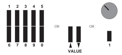
③ You can switch between User and Preset programs with Quad Knob [3]. By either pressing Quad Button [3] and then pressing VALUE [↑], or by turning Quad Knob [3] all the way to the right, the top line of the display will change to read "PROG TYPE: PRESET"
