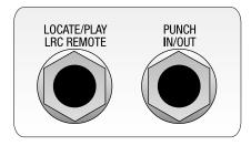
The two footswitch jack functions are designed to be used with any momentary single-pole/single-throw footswitch (either normally open or normally closed). These should be plugged in prior to power-up so that the XT20 can configure itself for the type of footswitch being used.
