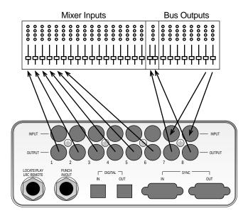
In addition, an external synchronizer connected to the XT20's [SYNC OUT] can output SMPTE or MTC to simultaneously synchronize a MIDI sequencer to tape. This way, you can mix down not only the first 6 tracks from the XT20 but your "virtual" tracks on the sequencer as well, all onto tracks 7 and 8.
