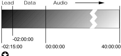
If an unformatted tape is not at the very beginning, it will automatically be rewound to the beginning. However, if any formatting is detected while rewinding, the transport will stop rewinding and leave the tape at this position, ready for a format extension (see next page).
