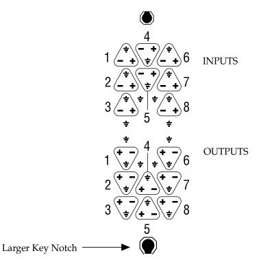
*Note:* The larger of the two outer key notches is at the bottom.
