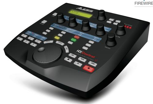
The io|Control is the ultimate interface and control surface for both mobile recording and home studio use. Backed by Alesis' unmatched reputation in the field of professional studio electronics, the io|Control allows for up to 12 channels (4 analog and 8 digital) of simultaneous input to your computer via the integrated, low latency FireWire interface.
