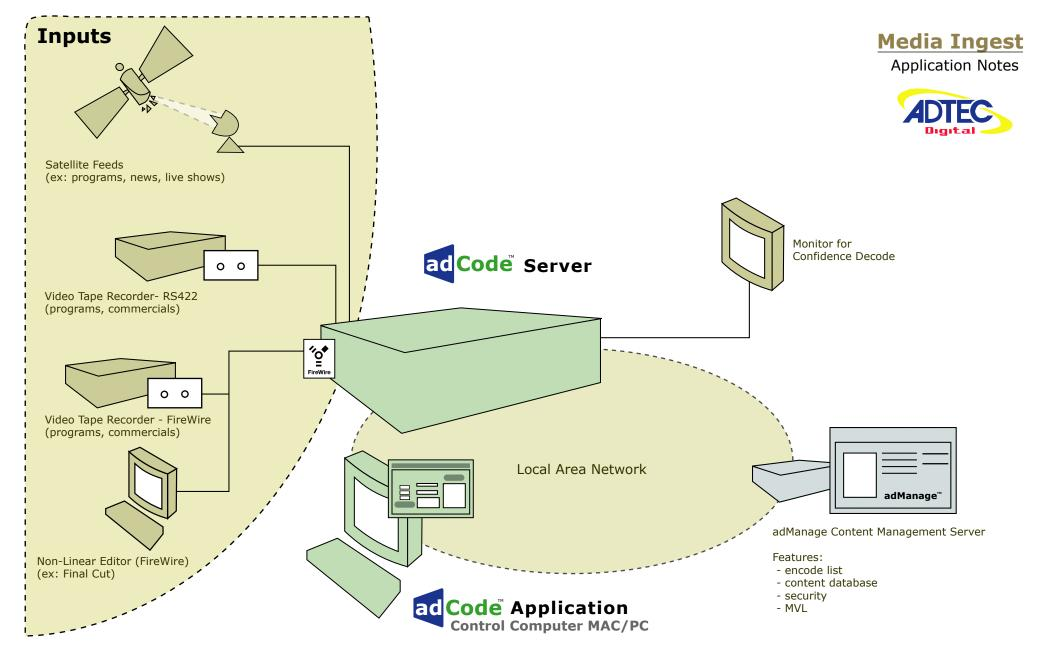
he adCode server and application combine to provide a media ingest station for MPEG 2 standard definition encode, review and approval of commercial and program material from FireWire (DV25), SDI, analog composite or YC sources. adCode includes control of professional VTRs over
