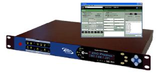
MediaHub Pro is Adtec's new media ingest encoder, It allows RS422 communications with VTR decks for precise encoding using mark-in and mark out features. Live feeds from studio or
