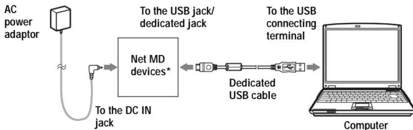
\* If a cradle is supplied with your Net MD, connect the dedicated USB cable to the USB cradle and place the Net MD onto the USB cradle.
