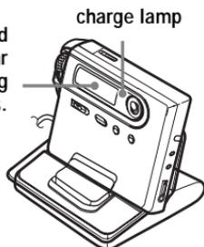
The remaining charging time appears in the display. The charge lamp will go off about one hour after you place the recorder on the USB cradle. At this point, the battery is about 80% charged. After 3 more hours, the battery will be fully charged.
