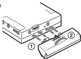
Insert a LR6 (size AA) alkaline dry battery.
