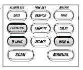
To cancel this function, press *HOLD* to hold the search and select the frequency by using *HOLD* or  $\checkmark$  *LIMIT*, then press *LOCKOUT*.
