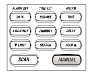
To select the channel (12), press 1, then 2 on the numeric keypad. Then press MANUAL again.
