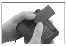
2) Insert the (2) "AA" batteries into the compartment as indicated in the drawing below. Be sure the negative (-) end is against the spring. Refer to the drawing below to insure correct installation of your batteries.
