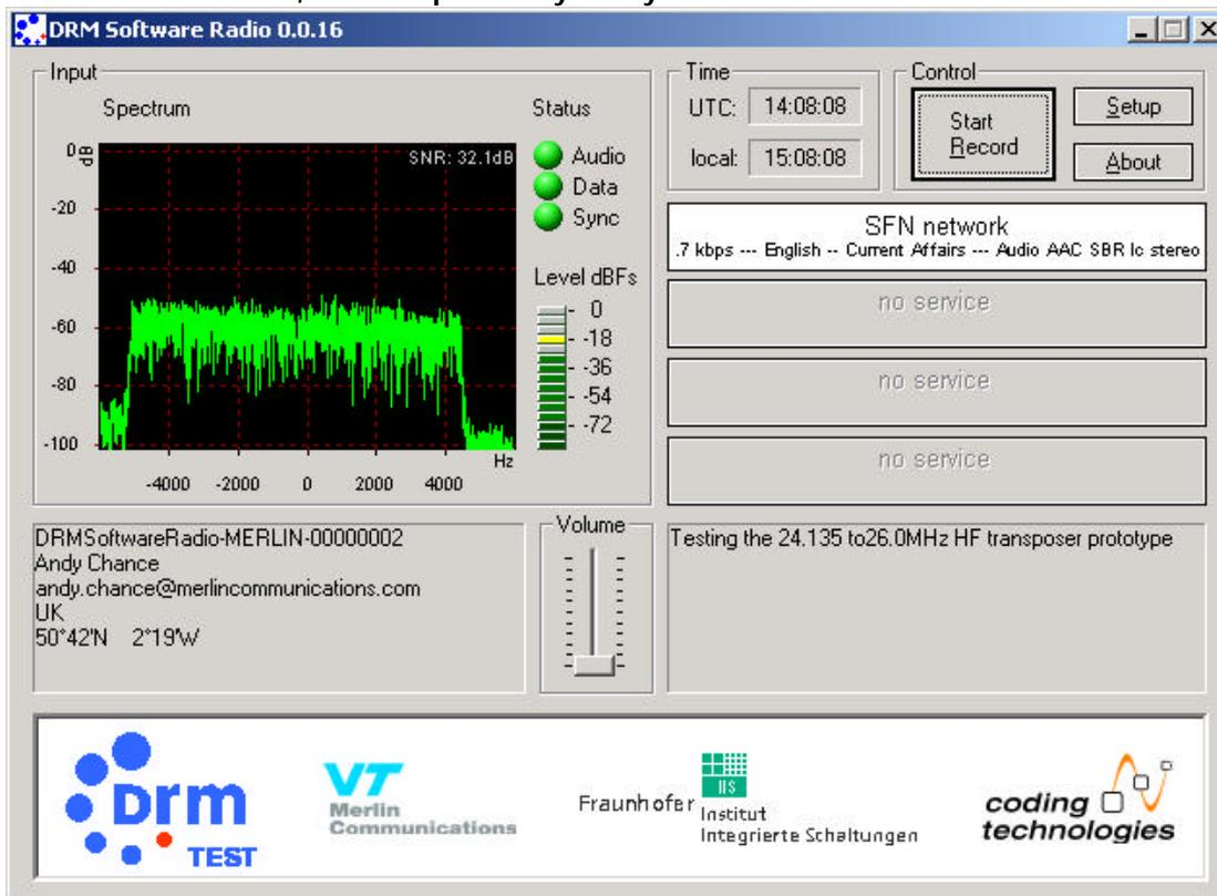
Note, both look very similar on the spectrum display but with very different SNRs. 20dB is just sufficient to decode the high data rate in use here.
