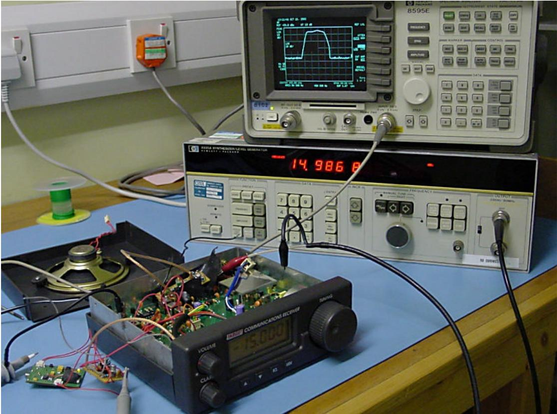
Testing with DRM signal. The 455kHz IF is displayed on the spectrum analyser.
