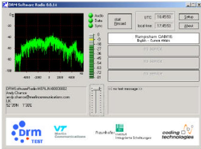
This screen shot of the software was taken of using the output from the AKD HF3. It works, but the input was a test generator! A better receiver would give a flat top and steep sides.
