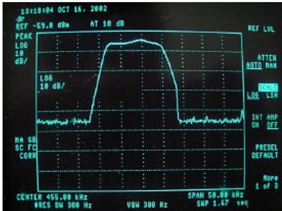
The response is significantly improved, but still shows some ripple and falls off a bit steeply at the high frequency end.
