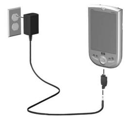
4. When the power indicator on the top of the iPAQ Pocket PC turns solid amber, the unit is fully charged and you can disconnect the AC Adapter. The approximate time to fully charge a unit is four hours.
