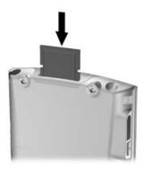
4. To prevent power loss, remove any expansion cards from the SDIO expansion slot before turning off the iPAQ Pocket PC. Leaving in the expansion card can drain the unit.
