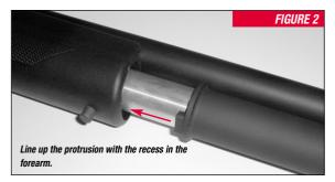
5. Insert the forward magazine sleeve onto the magazine tube, flanged end first. This is the end with the noticeable flange and a rectangular protrusion coming from the flange.
