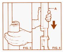
8. Replace the valve assembly back onto the magazine and turn until "hand tight".
