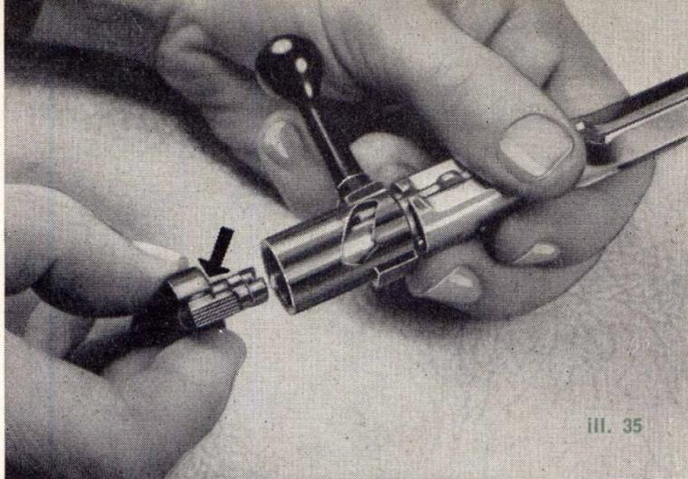
**JII. 36.** Withdraw the bolt-handle unit to the rearward. Here again, see that the spring pin (a) does not fall out. Hold the bolt horizontally.
