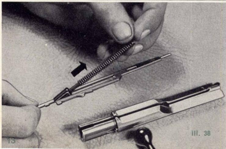
**III. 38.** Depress the striker spring and remove to the forward together with forked spring pin. The action is now completely dismantled.
