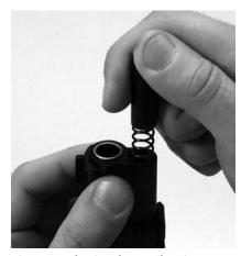
Figure 6: Releasing the recoil spring
