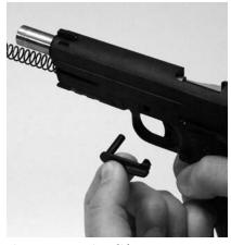
Figure 7: Removing slide stop
