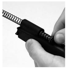
Figure 12: Insert recoil spring and guide into slide
