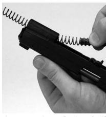
Figure 8: Removing recoil spring and guide
