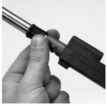
Figure 9: Removing bushing from slide
