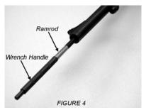
Note: Completely screw wrench handle into small end of ramrod until shoulder bottoms on brass end of ramrod.
