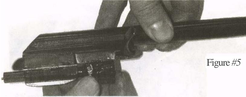
9. Remove the gas tube with the hand guard from the barrel. Holding the rifle by the forward portion of the receiver with the left hand, rotate the lock lever upward with the right hand, rotate the gas tube upward by means of the rear end of the receiver and remove it from the gas cylinder.
