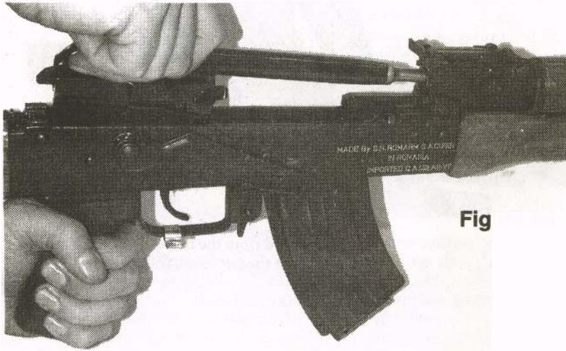
4. Install the return mechanism in the bolt carrier. Hold the rifle by the forward portion of the receiver with the left hand, and with the right hand insert the return mechanism into the bolt carrier channel, move the return mechanism rear face forward and placing its guide lugs opposite the grooves in the receiver rear plate, depress the return mechanism rear face, in this position, the rear faces should enter the groove in the receiver rear plate.
