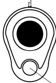
A smooth guide rod end means you have either a captive or a one-piece undrilled system, so...
