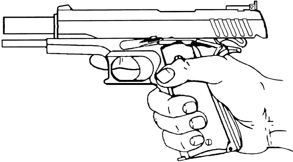
This feature tells the shooter that his pistol is empty, and permits rapid reloading. Press the slide stop down out of its locking notch to allow the slide to move forward. If a loaded magazine is inserted and the slide stop is pushed down, the slide will load a fresh cartridge from the magazine into the chamber, and the pistol is ready to fire.
