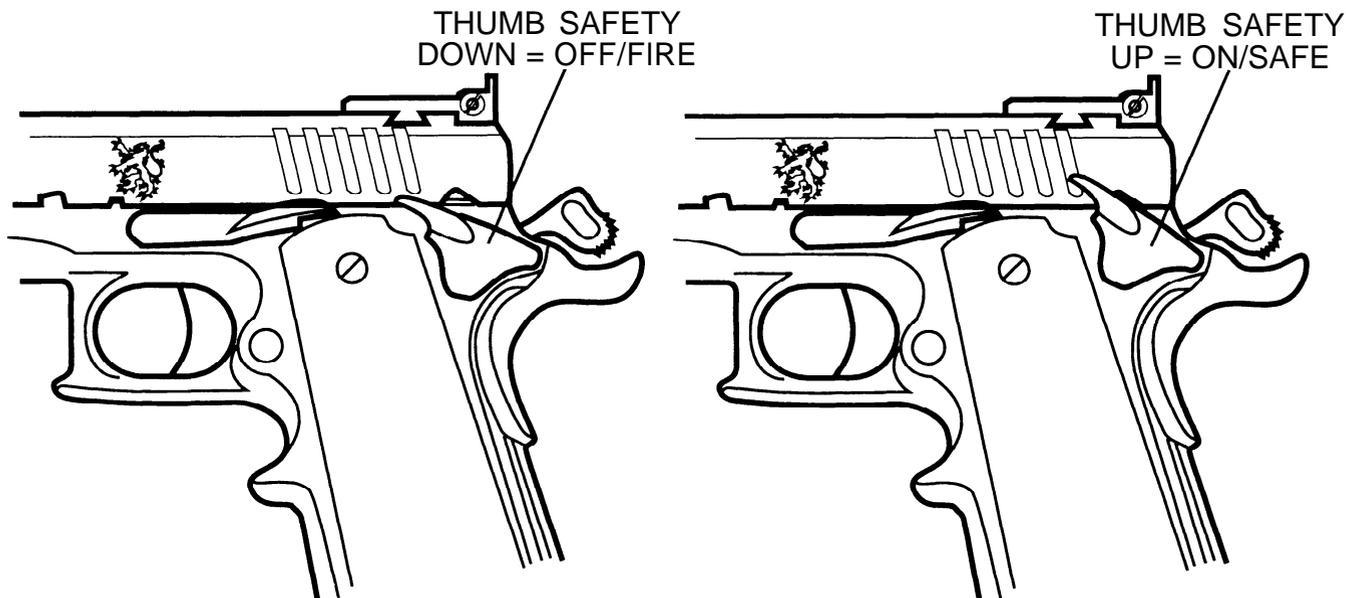
with the hammer down on an **EMPTY CHAMBER**. This allows a loaded magazine to be safely inserted into the pistol.
