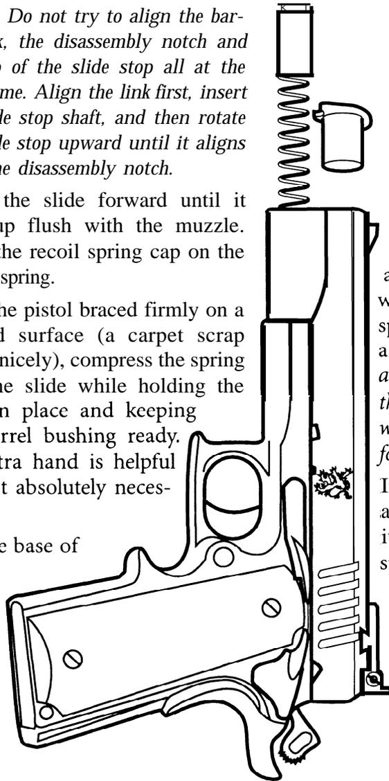
a magazine or a barrel bushing wrench to compress the recoil spring cap flush with the slide and muzzle. *Keep the muzzle aimed away from your face – if the spring gets away from you it will shoot out with considerable force.*
