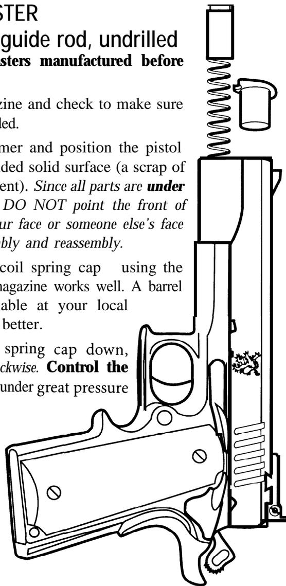
Move slide back until take-down notch is above slide stop tab.
