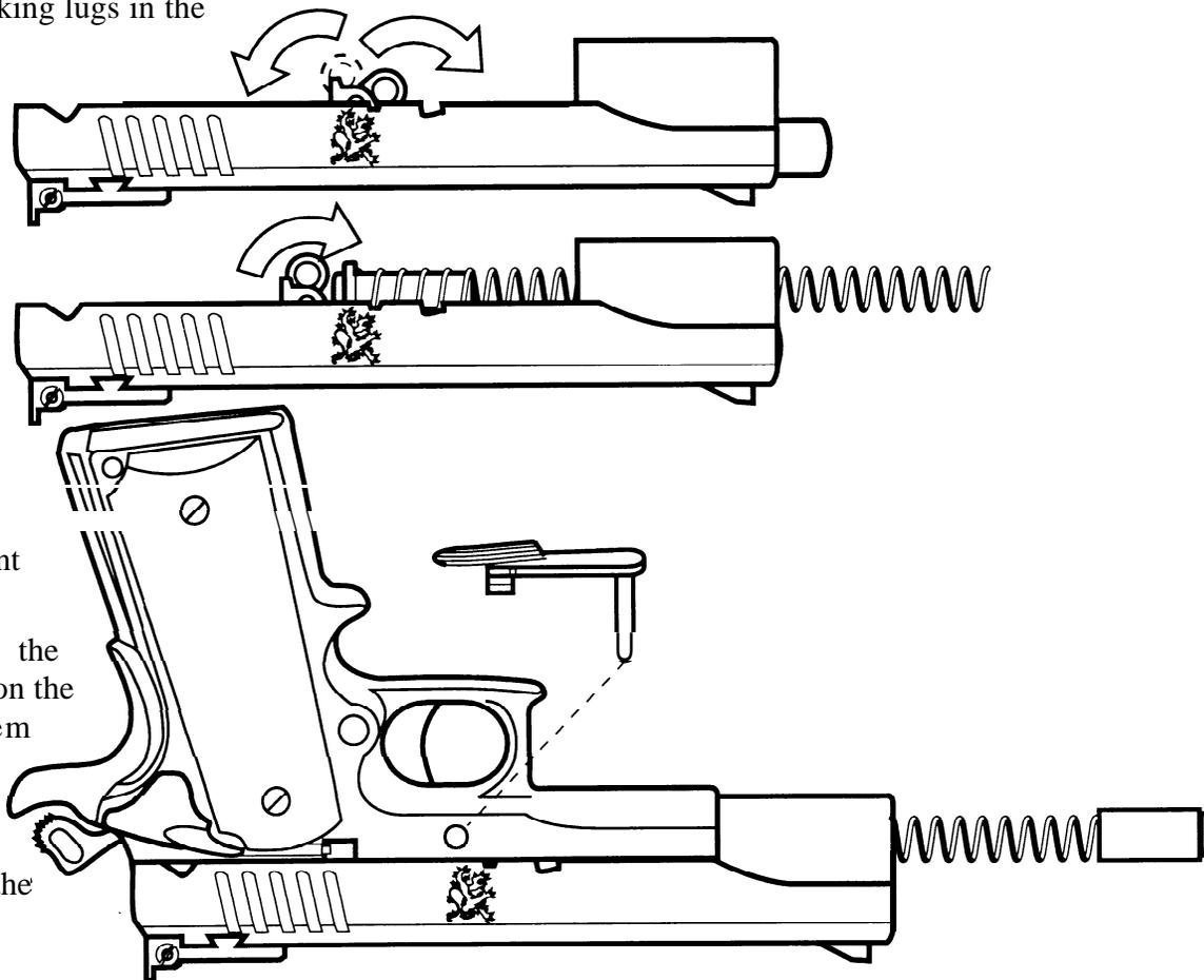
*NOTE: Do not try to align the barrel link, the disassembly notch and the top of the slide stop all at the same time. Align the link first, insert the slide stop shaft, and then rotate the slide stop upward until it aligns with the disassembly notch.*
