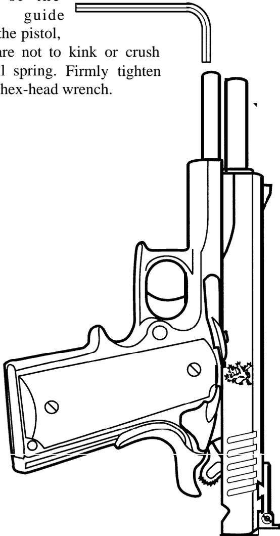
Move the slide to the rear until the slide stop lines up with the slide stop notch.
