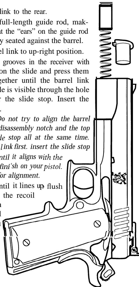
With the pistol braced firmly on a padded surface (a carpet scrap works nicely), compress the spring into the slide while holding the slide in place and keeping the barrel bushing ready. About this time you'll wish you had a third hand.
