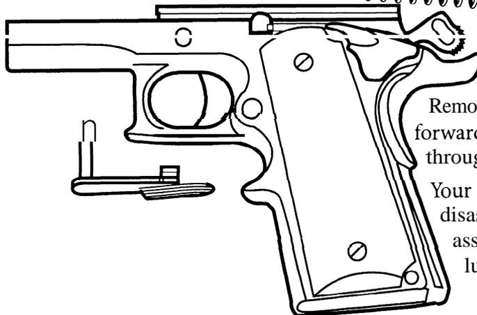
Then twist the barrel bushing counter-clockwise and remove.
