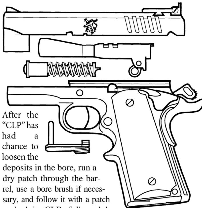
After the “CLP” has had a chance to loosen the deposits in the bore, run a dry patch through the barrel, use a bore brush if necessary, and follow it with a patch soaked in CLP, followed by another dry patch.
