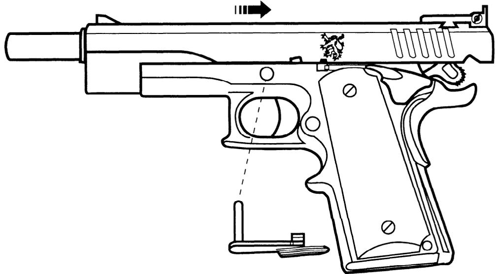
Ease the slide forward into battery. Then, while gripping the slide and receiver, move the slide forward off the receiver. Maintain your grip on the slide and its internal components (barrel and recoil unit) to keep them from springing apart.
