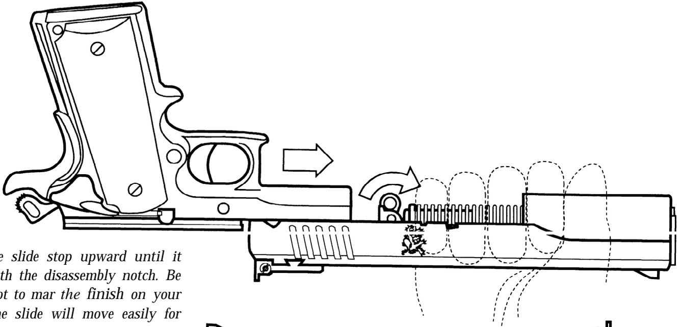
*rotate the slide stop upward until it aligns with the disassembly notch. Be careful not to mar the finish on your pistol. The slide will move easily for alignment.*
