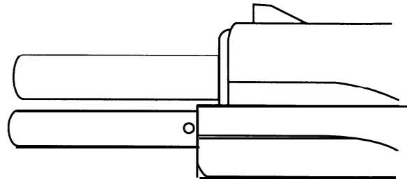
move the slide back until the slide stop engages. Look at the guide rod. If there is a tiny hole drilled through it, you have a captive system (page 15). If there isn't, you have the undrilled system (page 26).
