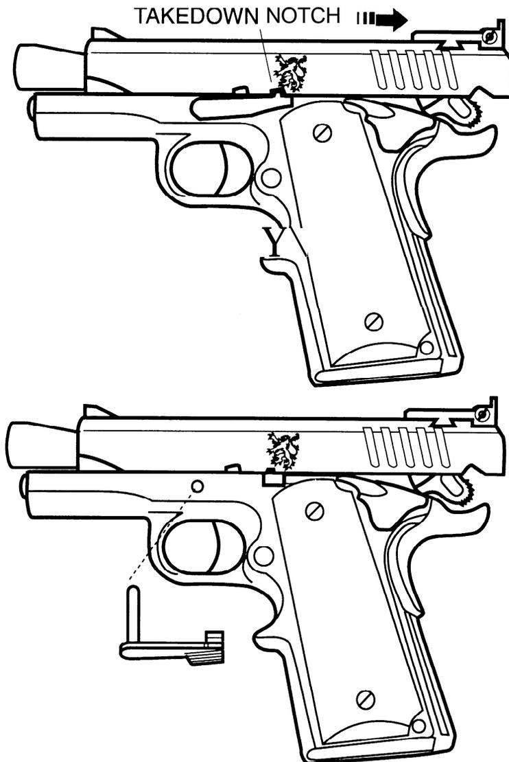
Remove slide unit by moving it forward and off the frame.
