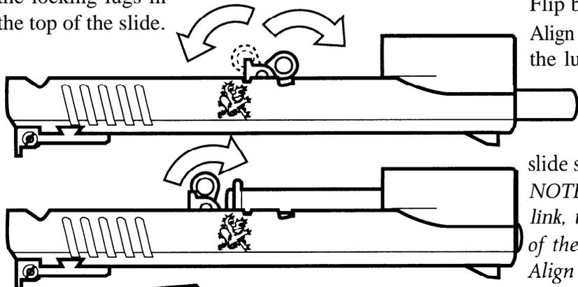
shaft, and then rotate the slide stop upward until it aligns with the disassembly notch. Be careful not to mar the finish on your pistol. The slide will move easily for alignment.
