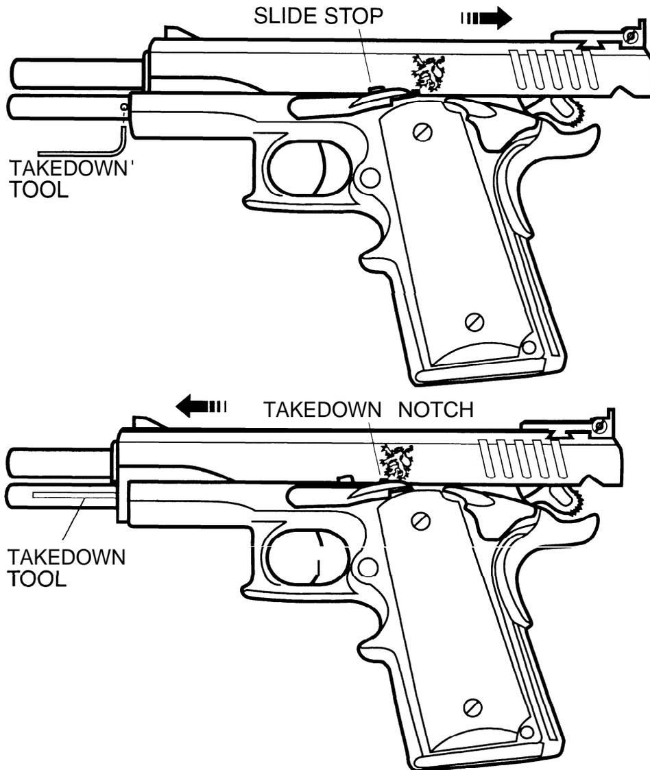
Remove the slide stop by pulling it straight out - it can be started by pressing on the end that protrudes from the opposite side of the frame.
